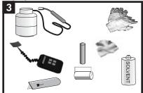
Propane tank, hose, torch & regulator Appropriate tools for surface abrasion Knife, roller, rags & approved solvent cleanser Digital thermometer with suitable probe Standard safety equipment; gloves, goggles, hard hat, etc.
