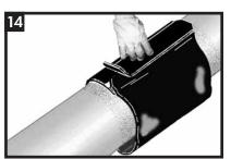
Remove any release liners from the Closure Strip Centre the closure on the overlapping sleeve. Press down firmly.
