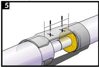
Drill one foaming hole over the pressure testing hole. Drill the other foaming hole, if required (as close to the shrinkable end as possible while remaining in the cutback area).
