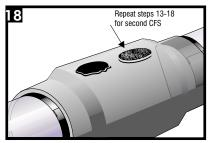
The CFS has been fully installed when adhesive can be seen around the entire circumference.
