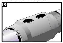
The CFS has been fully installed when adhesive can be seen around the entire circumference. Visually inspect that the patch for any breaks or holes.
