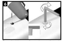
Foam the joint according to the manufacturer's guideline using standard foaming plugs to seal the foam holes.
