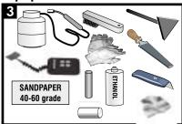
Propane tank, hose, torch & regulator Sandpaper (40-60 grade) or wire brush Knife, roller, rags & ethanol (min. 94%) cleanser Temperature measuring device, grater, triangular scraper Standard safety equipment; gloves, goggles, hard hat, etc.
