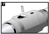
Using a roller and a gentle flame, smooth out the CFS surface.
