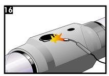
Using a medium flame, heat the backside of the CFS until the adhesive oozes from the edge of the patch.
