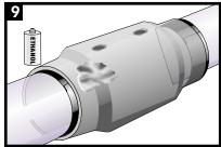
De-grease the surface of the casing using a grease and lint-free rag soaked in ethanol.
