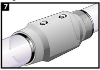
After the foam has hardened, remove the foam plugs and weld the standard weldable plugs.
