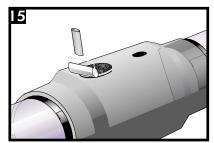
Using a gloved hand or roller, pat down the CFS for about 5 seconds, or until the entire CFS surface makes good contact with the casing.
