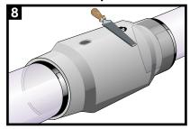
Using a grater, sand down the plugs bringing them flush to the surface of the casing.
