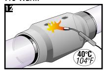
Pre-warm the casing surface around the foaming hole to 40°C. Check the temperature using a temperature measuring device.
