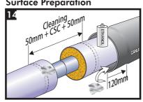
Clean the surface of the jacket pipe and the inside of the thin shrink zone of the casing with a rag to remove dirt. Degrease the surface of the jacket pipe and the inside of the CSC using a grease and lint-free rag soaked in ethanol (min. 94%) or isopropyl alcohol cleanser.
