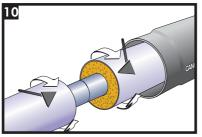
Using a triangular scraper, clean the edges of the jacket pipe to remove any burrs and dirt from the sealing area.
