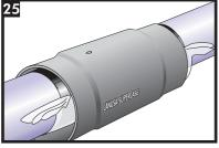
Completely remove the release liners from the adhesive strips.
