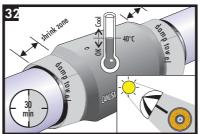
Allow the CSC to cool for 30 minutes. After 30 minutes measure the surface temperature of the CSC shrink zones. If the surface temperature of the shrink zones are still above 40°C, use shading and/or damp towels to quicken CSC shrink zone cooling time.
