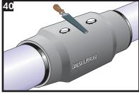
Using a grater, sand down the plugs bringing them flush to the surface of the CSC.
