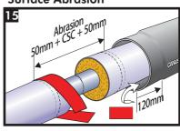
Roughen the surface of the jacket pipe on both sides of the cutback and the **inside of the CSC** (thin shnink zones) using the sandpaper (40 to 60 grade).
