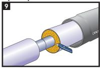
Remove any wet PUR foam from the end of the pre-insulated pipe.
