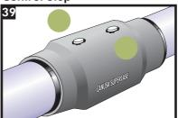
Continue with step 39 when the foaming hole is to be double sealed with a weldable plug and Canusa Foam Seal - CFS.
