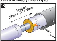
$\begin{array}{l} \label{eq:pre-warm the pipe to 40°C-50°C. \\ \hline \textbf{Ensure the correct temperature with a temperature measuring \\ \textbf{device.} \quad Do not exceed 60°C as this makes the removal of release liner difficult. \end{array}$
