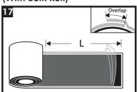
If not using the pre-cut adhesive from a kit, measure the circumference of the jacket pipe and cut two sealing strips long enough to allow for
