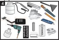
Propane tank, hose, torch & regulator Sandpaper (40-60 grade) or wire brush Knifer, roller, rags & ethanol (min. 94%) or isopropyl alcohol cleanser Temperature measuring device, triangular scraper Marking pencil, grater, drill, CFS Rolling Tool Standard safety equipment; gloves, goggles, hard hat, etc.
