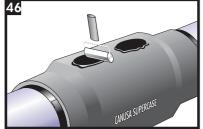
Using a roller, gloved hand or the side of the larger end of the CFS Rolling Tool; smooth out the CFS surface. Ensure adhesive has oozed from all sides of the CFS.
