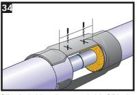
Drill one foaming hole over the pressure testing hole. Drill the other foaming hole, if required (as close to the shrinkable end as possible while remaining in the cutback area).
