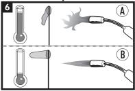
Adjust the flame according to outside conditions. a. Use bluish-yellow flame for low wind, higher temps b. Use blue flame for high wind, lower temperatures Always aim the torch perpendicular to the shrink zone of the CSC and move in a circumferential direction.
