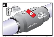
De-grease the surface around the plug using a grease and lint-free rag soaked in ethanol.
