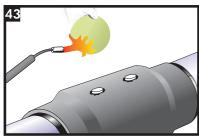
Heat the adhesive side of the CFS with a medium intensity flame until the adhesive becomes clossy (Adhesive will melt).
