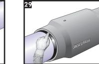
As a final check, ensure that the shrink zone of the CSC conforms intimately with the entire pipe surface. This can be checked by feeling the edges all around the circumfreence of the casing. If there is edge lifting, the edge should be reworked with additional heat.
