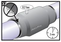
Ensure the CSC shrink zones have cooled to below 40oC. Perform the pressure test using the previously drilled pressure hole. The CSC should be checked with an air pressure test for 3 minutes at 0.2 bar. In case of a leak, the CSC shrink zones should be reworked with additional heat at the leaking area. The pressure test should then be repeated.
