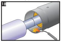
Pre-warm the inside of the casing on each end (150mm) by moving it half-way over the joint. Use low intensity flame to make sure that the casing does not start to recover.
