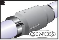
For casing sizes PE355 and above, wrap the supplied tension tape around the edge immediately after shrinking, while the casing is still soft (if the casing has cooled down; reheat it). **This ensures even cooling and conformance of the edges.**
