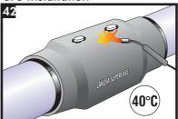
Pre-warm the casing surface around the foaming hole to 40°C. **Do** not overheat the surface as the foam will gas. Check the temperature using a temperature measuring device.
