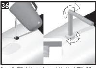
Ensure the CSC shrink zones have cooled to at least 40°C. If they have not, follow the cooling instructions as described in step 31 (for CSC 560 and greater, follow steps 31 and 34). Do not foam if the surface temperature is above 40°C. Foam the joint according to the manufacturer's guideline. Use standard ventilation plugs while foaming. After the foam has cured, remove the foaming straps (if used).
