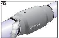
With a gloved finger, press down on the shrunk area to ensure the backing and adhesive are soft. If there are cool spots, the shrink zone should be reworked with additional heat.
