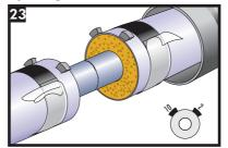
Remove the paper backing and place the spacers at the 10 and 2 o'clock positions of the jacket pipe, right at the edge of the cutback.
