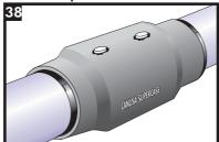
Visually inspect the completed casing. Ensure that the ends of the CSC are completely shrunk down. To double seal the foaming hole use a Canusa Foam Seal - CFS.
