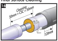
Using a dry, grease and lint-free rag, clean the roughened surface to remove any polyethylene or sand particles.
