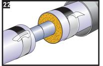
Fold the release liner outwards to allow for easy removal after positioning the casing.
