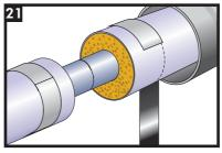
...apply the adhesive strips tightly around the jacket pipe with the mesh side facing up. The strips should be applied so that they are placed approximately 5mm inside of the marks. Make sure the adhesive is not stretched during wrapping. Partially peel-back the release line on the under lap and wrap the strips around the jacket pipe so that they overlap.
