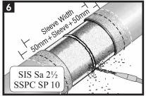
Warm the joint area to 40-50°C (100-120°F) before grit blasting. Thoroughly clean the weld area with a sand or grit blaster to "near white metal" SIS Sa 2½ or equivalent. Abrade the mainline coating adjacent to the weld area to a distance 50mm (2") beyond the sleeve width.
