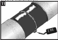
Check the temperature to ensure the preheat has been obtained on the entire pipe circumference. This preheat will substantially cure the epoxy and ensure proper flow and bonding of the sleeve adhesive. Ensure that the epoxy primer is dry to the touch prior to sleeve installation. installation.
