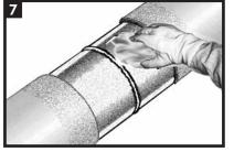
Using a dry, grease and lint-free cloth, wipe clean or air blast the steel and coated areas to remove foreign materials. If necessary, provide additional heat to ensure the surface temperature is  $40-50^{\circ}$ C ( $104-120^{\circ}$ F).
