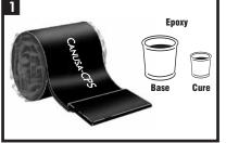
GTS-65 Global Transmission Sleeves are shipped pre-cut with a pre-attached closure. Butk quantities are also available. The sleeve adhesive is protected from contamination by an inner liner. The joint completion system may also use an epoxy primer.
