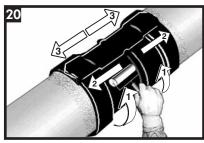
While the sleeve is still hot and soft, use a hand roller to gently roll the sleeve surface and push any trapped air up and out of the sleeve, as shown above. Continue the procedure by also firmly rolling the closure with long norizontal strokes from the weld outwards.
