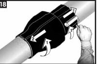
While the sleeve is still hot and soft, use a hand roller to firmly roll the sleeve surface and push any trapped air up and out of the sleeve, as shown above. If necessary, reheat to roll out air.
