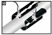
Wrap the WLOX sleeve around the tyton joint. Gently heat the backing of the underlap and the adhesive side of the overlap. Finish wrapping the sleeve around the tyton joint pressing the overlap firmly into place.
