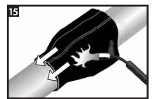
Continue shrinking from the bell of the tyton joint to the sleeve end. Sleeve recovery is complete when it sleeve end. Sleev conforms to the pipe.
