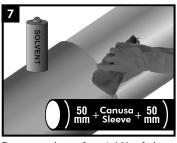
De-grease the surface (width of sleeve + 50 mm on each side) using a grease and lint-free rag soaked in ethanol (min. 94%) or other suitable solvent.
