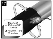
Using the appropriate torch, begin at the centre of the sleeve and heat circumferentially around the pipe. Use broad strokes. If utilizing two torches, operators should work on opposite sides of pipe.
