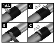
Gently heat the closure and pat it down with a gloved hand. Repeating this procedure, move from one side to the other. Smooth any wrinkles by gently working them outward from the centre of the closure with a roller or by patting the closure down.
