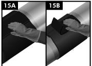
Pre-cut sleeves with pre-attached closure: Press the closure firmly into place. Bulk Sleeve Roll with separate closure: Center the closure over the overlap and press it down
