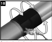
Continue heating from the centre toward one end of the sleeve until recovery is complete. In a similar manner, heat and shrink the remaining side.
