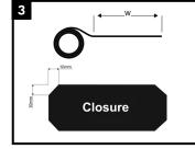
Cut the required length (W) of closure material from the bulk roll. Closure (W=sleeve width less 5mm)
