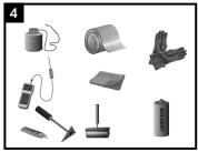
Propane tank, hose, torch & regulator Appropriate tools for surface abrasion: 40-60 grade sandpaper, knife, roller, triangular scraper, rags & approved solvent cleanser Digital thermometer with suitable probe Standard safety equipment; gloves, goggles, hard hat, etc.
