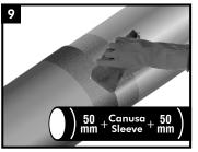
Clean the roughened surface to remove any polyethylene or sand particles, using a dry grease and lint-free rag.
