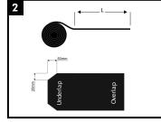
Cut the required length (L) of sleeve material from the bulk roll. SuperSeal<sup>™</sup>- B (L=circumference of casing + 120 mm)
