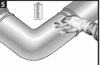
Ensure that the PE coating edges are beveled to  $30^{\circ}$ . Clean exposed steel and adjacent pipe coating with a solvent cleanser to remove the presence of oil, grease, and other contaminants.
